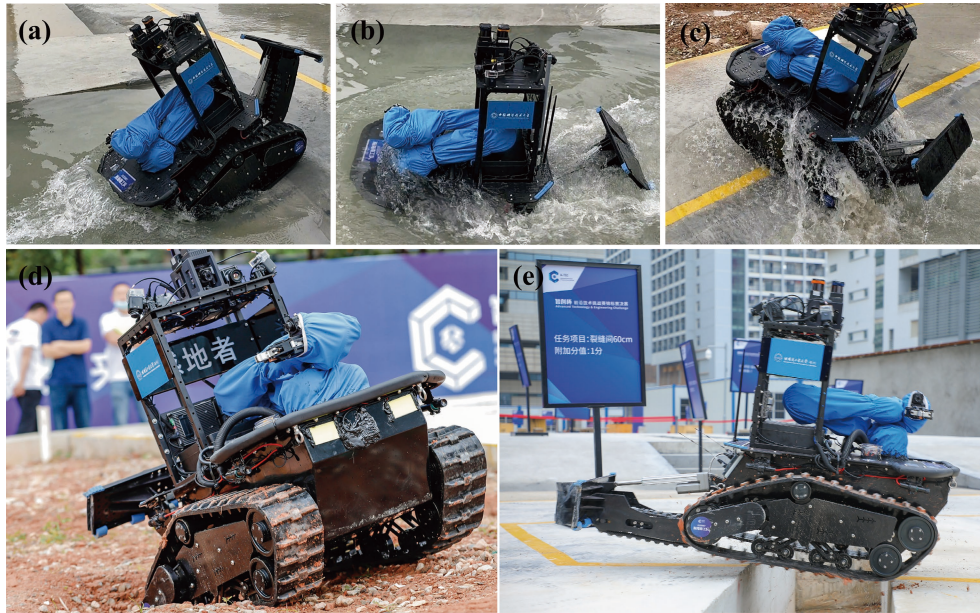
Fig. 6. Snapshots of Earthshaker in Session 1. (a)–(c) Earthshaker was passing through a pool filled with water of 500 mm in depth. (d) Earthshaker was traversing muddy terrains. (e) Earthshaker was crossing a trench of 600 mm in width.
