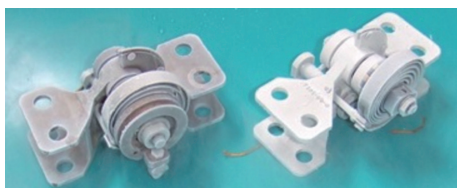
Fig. 10. Picture of function test for hinges after storage in LN for one year.
