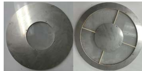
Fig. 2. Mesh 1 and Mesh 2 used to bias two plasma layers.
