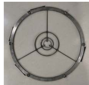
Fig. 3. Ring electrode designed to modulate the distribution of plasma potential.
