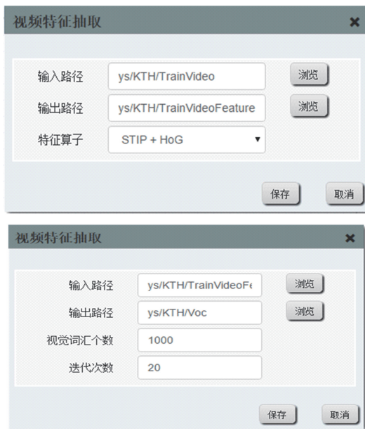
图 14 特征抽取和视觉词汇生成配置面板 Fig.14 Feature extraction and visual vocabulary generation configuration panel
